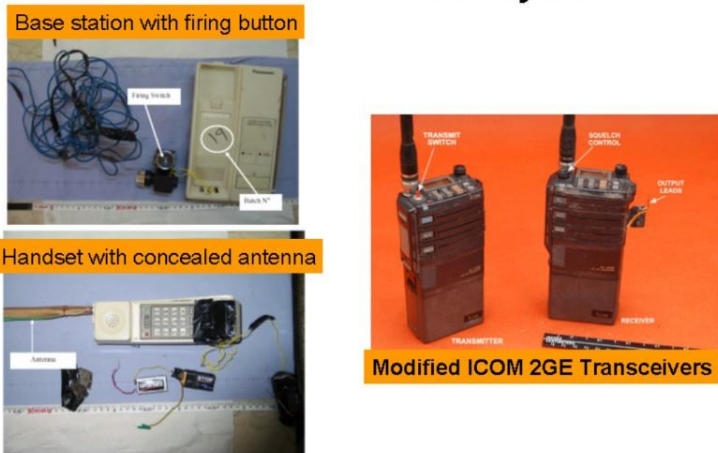
Рис.15. Радиоуправляемое СВУ(Radio Controlled Improvised Explosive Device).
